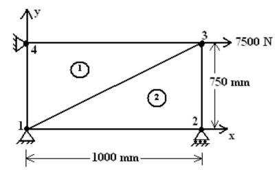
3. A thin plate is subjected to surface traction as in figure. Calculate the global stiffness matrix.
