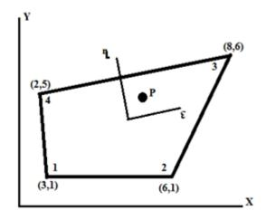
4. A four noded rectangular element is in figure. Determine (i) Jacobian matrix, (ii) Strain – Displacement matrix and (iii) Element Stresses. Take  $E=2x10^5 N/mm^2$ , v=0.25,  $u=[0,0,0.003,0.004,0.006, 0.004,0,0]^T$ ,  $\xi=0$ ,  $\eta=0$ . Assume plane stress condition.
