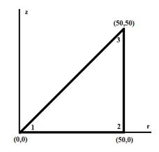
2. For the figure, determine the element stresses. Take  $E=2.1 \times 10^5 N/mm^2$  and v=0.25. The co – ordinates are in mm. The nodal displacements are  $u_1=0.05mm$ ,  $w_1=0.03mm$ ,  $u_2=0.02mm$ ,  $w_2=0.02mm$ ,  $u_3=0.0mm$ ,  $w_3=0.0mm$ .
